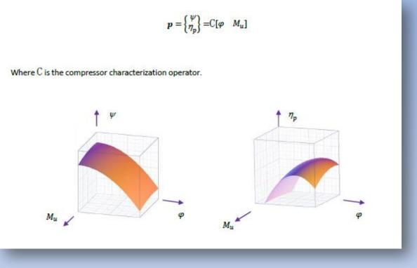
compressor model is characteristic of the machine and represents the invariant base of information upon which it is possible to build the predictions of the compressor performances in operative conditions different from the reference ones
