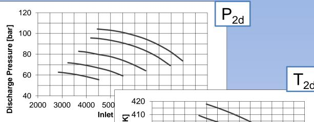
Usually compressor performance are known as set of curves of dicharge pressure and discharge temperature as function of inlet volume flow, each set includes many curves each one for a different running speed
